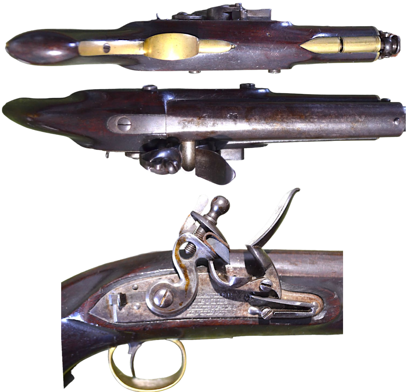
A. 65" FLINTLOCK PATTERN 1829 CUSTOMS / COASTGUARD PISTOL BY BARNETT CIRCA 1830, 4 ½" London proofed barrel with top flat, swivel rammer hinged to muzzle, Paget style bevelled, stepped and bolted lock with makers name 'BARNETT', raised semi waterproof pan, roller to frizzen spring, ring neck cock, full stocked with regulation style brass mounts. The first mention of this type of pistol occurs in official records in 1829 and is described as the 'Pattern of Short Pistol for Revenue Service', cost of manufacture is given as £1.10.00. Identical pistols together with short muskets for the Customs were also obtained from Barnett, see 'Arms of the Customs Service by H. L. Blackmore'. Journal of the Arms & Armour Society, September 1996, where similar pistols are illustrated and detailed. In very good condition with good stock, small chip toe leading edge of left forend, barrel rebrowned showing the attractive twist pattern. (92/24) £695
